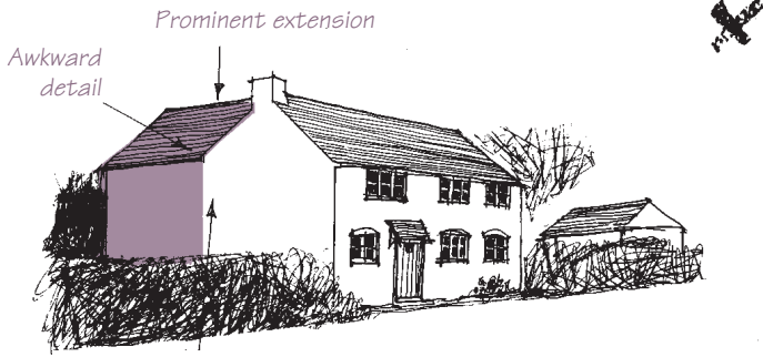
Difficulty in keying new brick work
