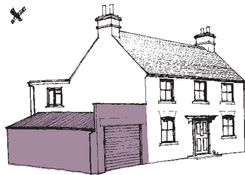
The use of parapets is not encouraged. A preferred arrangement for pitched roofs is similar form to the main roof
