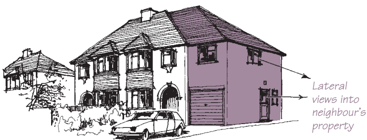
New openings on flank elevations can lead to problems of overlooking
