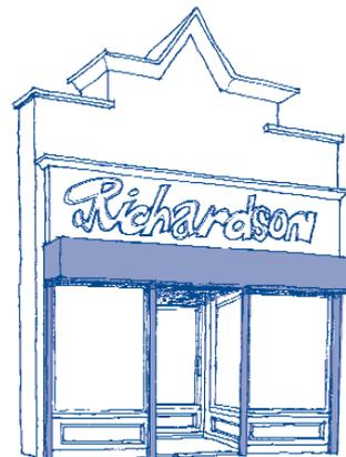
Recessed entrances add interest to shop fronts. Hidden grilles can be installed that allow the recess to be closed when the shop is shut.
